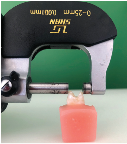
Fig. 1: Recording baseline measurement before the cavity preparation
