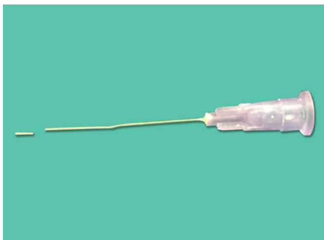
Fig. 5: A fractured irrigating needle along with the retrieved segment
