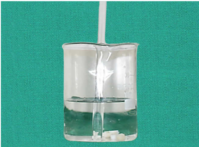
Fig. 8: Samples were immersed in a 1% citric acid solution
